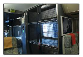
and the fact that they can be stored in a secured location – end coach rack and or overhead luggage compartment, locations designed to hold luggage and secure stored luggage in the event of an accident. Photo above shows VIA Rail end coach secure luggage location. <sup>11</sup>
